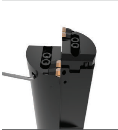
Step 2: Set one cartridge to the finish diameter by tightening the adjustment screw against the adjustment pin.
