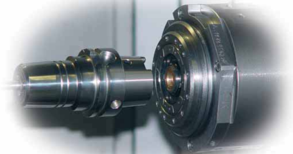
Fig. 1: HSK-A 63 interface, automatic tool change
